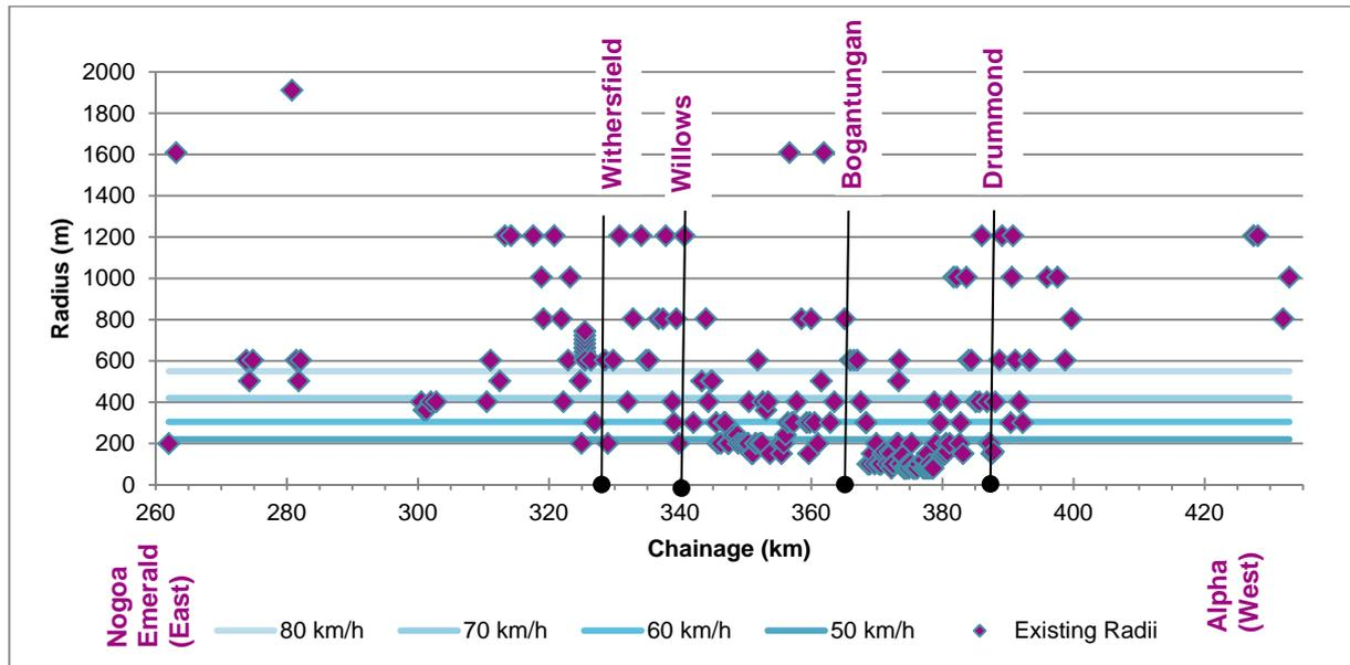
Figure 5 Existing radii against criteria limits for various speeds
