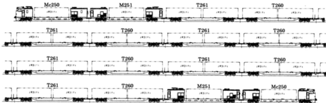
Figure 37 M250 Contrainer EMU: Extract from “Development of Super Rail Cargo” by Morita et al Japan Rail Freight Company
