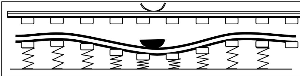
**Figure 18** Existing track structure mechanism with rails as main beam
