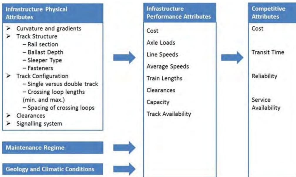
**Figure 9** The conventional link between infrastructure and service
