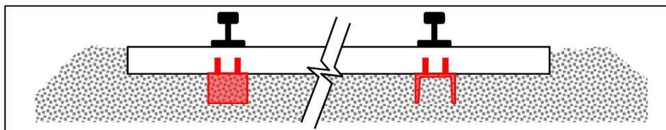
**Figure 19** Ideal supplementary beam under sleeper under rails
