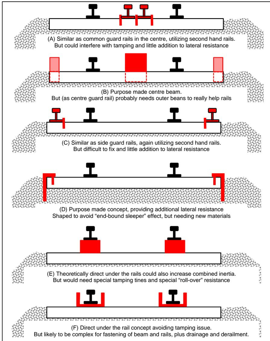
**Figure 20 Alternatives for supplementary beam positions and arrangements**
