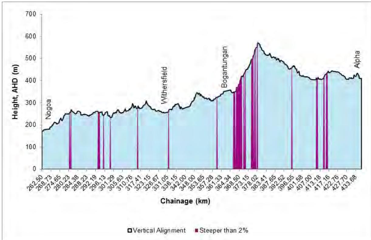
Figure 7 Existing vertical alignment and location of grades steeper than 2%
