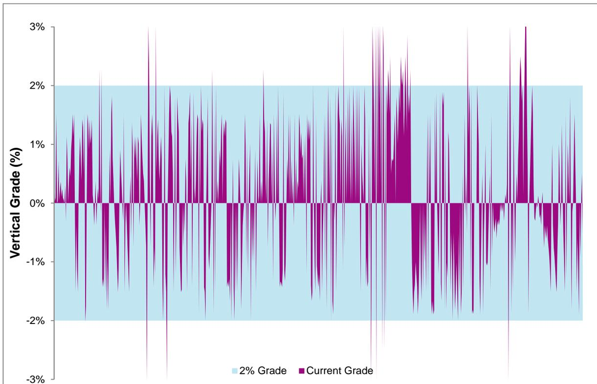
Figure 8 Comparison of existing grades and 2% (desirable) grade
