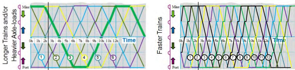
**Figure 30** Increase capacity through-put options <sup>37</sup>
