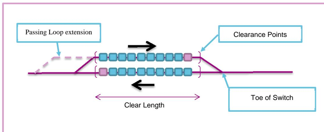
**Figure 9 Example Passing Loop**
