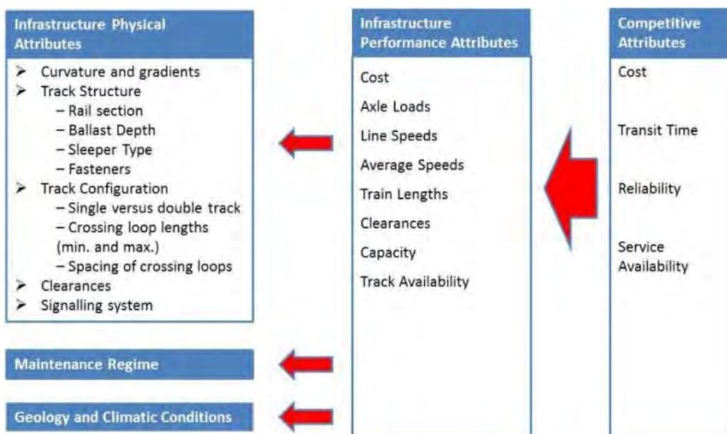
**Figure 10** Customer focussed service specification and infrastructure provision
