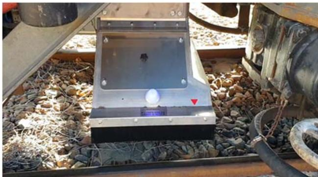
Figure 10 Condition Based Maintenance (CBM) – Example of output from the Rail Wear Analyser
