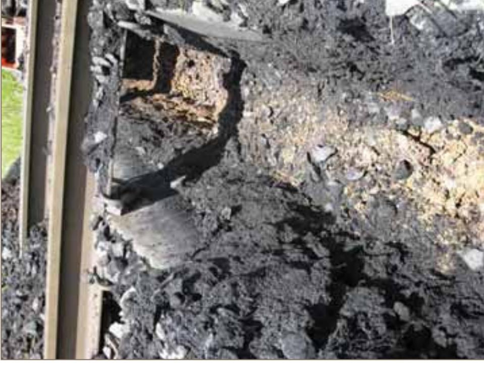
Sampling of Ballast by Destructive Means
