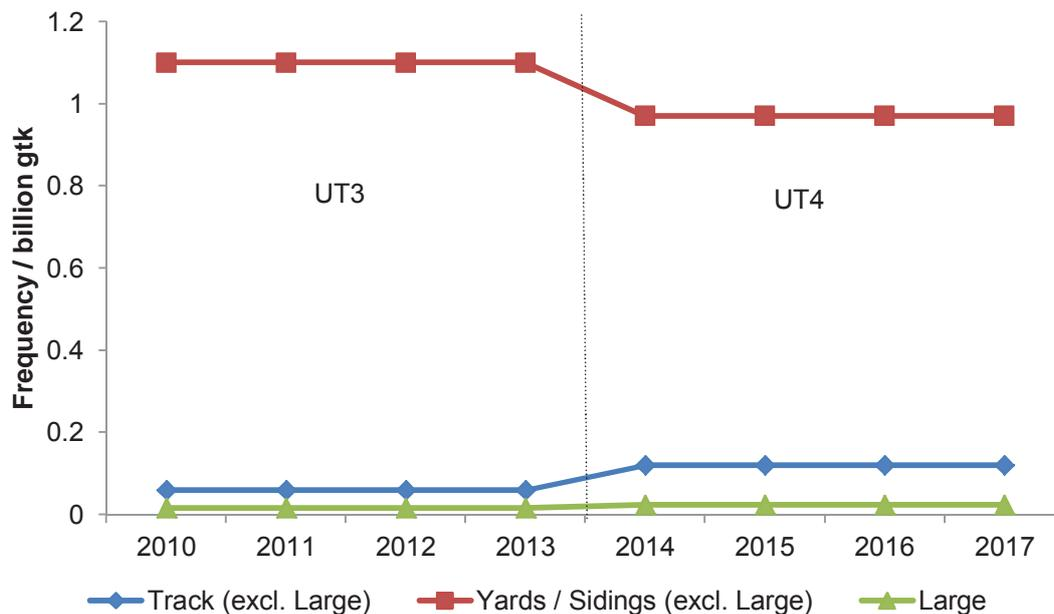
Figure 1 Aurizon Network's forecast derailment frequencies
