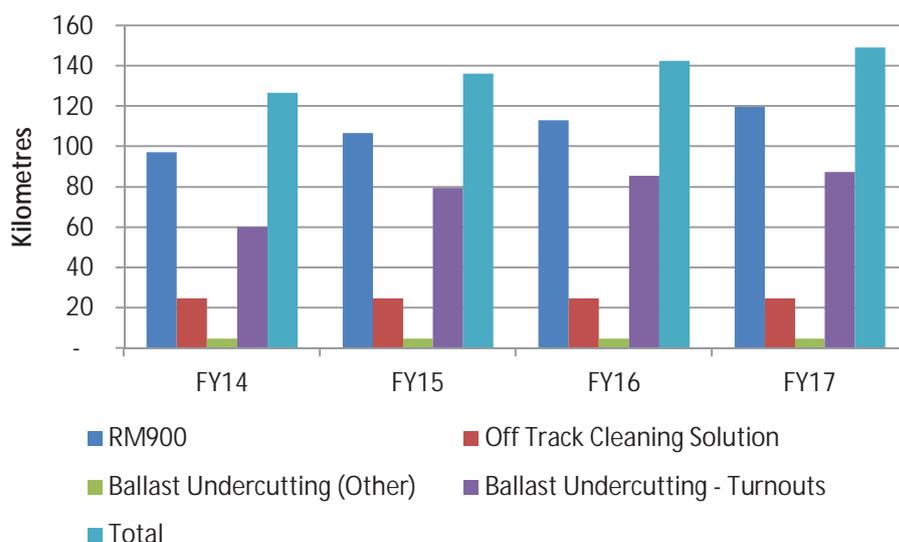
Figure 2.13 Aurizon Network's planned ballast undercutting scope
